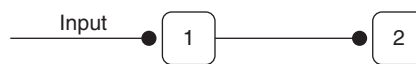
FIGURE 27.4 The smallest network, consisting of two cells driven by two excitatory conductances.
