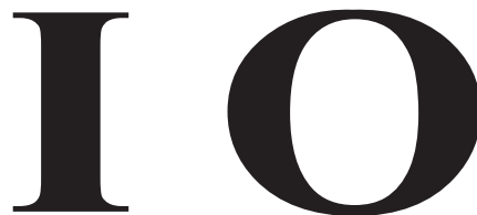
FIGURE 27.1 Binary visual patterns to be learned by a Hopfield network. Each of these letters is comprised of a 67-by-71 rectangular field of pixels, where black = 1 and white = -1. (hop.m)
