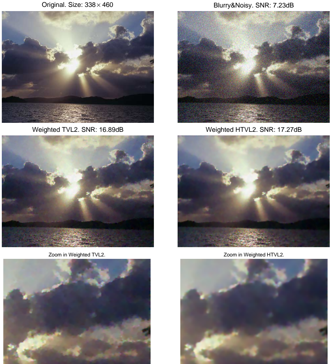
FIG. 4.5. Numerical results of weighted high order regularization. Original (upper left); Blurry and noisy (upper right); Weighted TV/L^2 result (middle left); Weighted higher-order result (middle right); Zoom in the results of weighted TV/L^2 (bottom left) and HTV/L^2 (bottom right).
