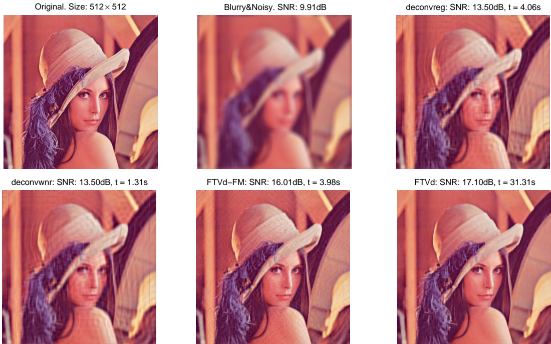
FIG. 4.2. Comparison results with MATLAB deblurring functions.
