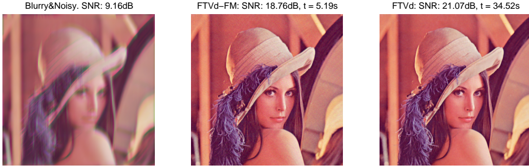
FIG. 4.3. Results recovered by FTVd-FM and FTVd from cross-channel blurring.
