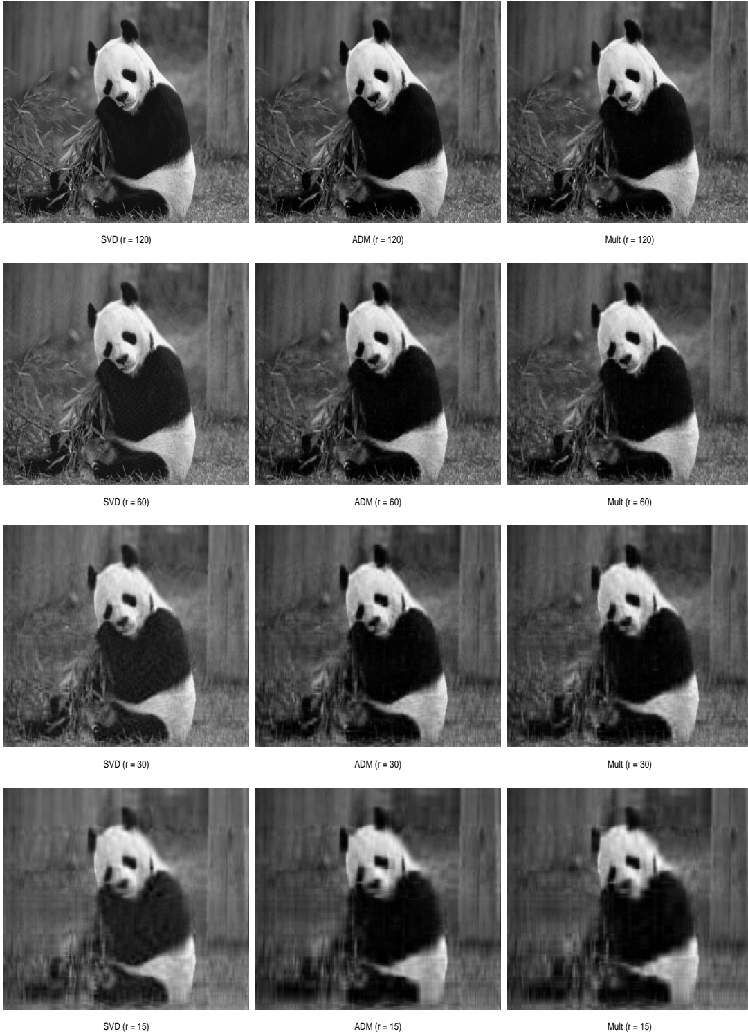
Figure 3: Results on the 1200 \times 1600 image Panda for rank k = 120, 60, 30, 15 (top to bottom) and for algorithms SVD, ADM and Mult (left to right).
