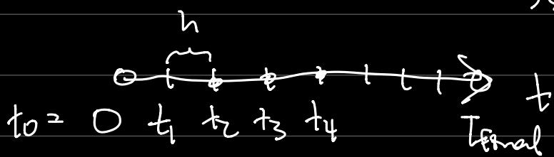
$$t_{k+1} = t_k + h \quad \vec{x}_0 \approx \vec{x}(t_0) = \text{initial condition.}$$
