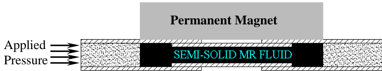
FIG. 18. Region of Bypass Duct Varying in Cross-Section
