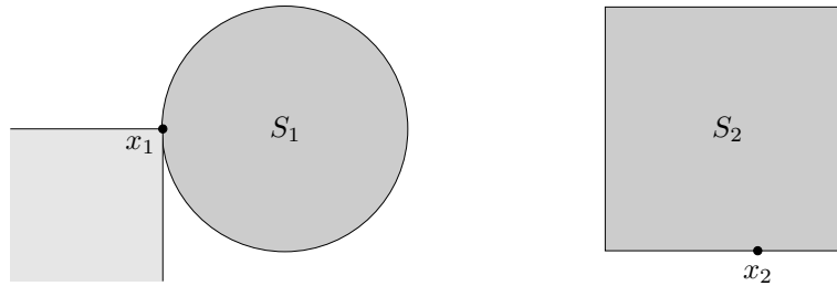
Figure 2.26 Left. The point x_1 \in S_1 is minimal, but is not a minimizer of \lambda^T z over S_1 for any \lambda \succ 0 . (It does, however, minimize \lambda^T z over z \in S_1 for \lambda = (1, 0) .) Right. The point x_2 \in S_2 is not minimal, but it does minimize \lambda^T z over z \in S_2 for \lambda = (0, 1) \succeq 0 .
